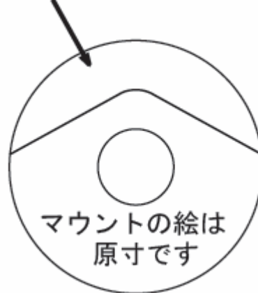
Motor mount (polypropylene make)
